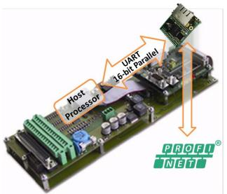
interfacing the Host processor to the UART or 16-bit Parallel interface. The Ethernet physical interface is ready to plug into the network. Software for the module is provided as firmware that is resident on the flash.
